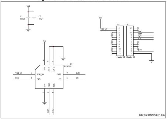
Figure 1. STEVAL- MKI142V1 circuit schematic
