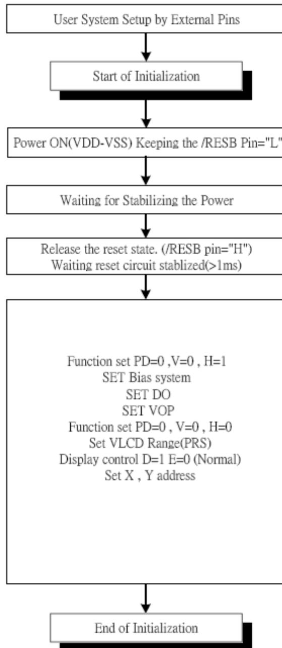
Initializing with the Built-in Power Supply Circuits
