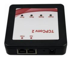
TCPConv 2 allows connecting a device with USB- or RS232-interface to an Ethernet network. A typical application is the extension of a network device (e.g. a network printer) by a local peripheral device.
