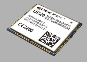
UC20 is the latest Quectel UMTS/HSPA+ module offering a maximum data rate of 14.4Mbps downlink and 5.76Mbps uplink. UC20 is designed to provide customers with global network coverage on the connectivity of UMTS/HSPA+. It can also be fully backward compatible with existing EDGE and GSM/GPRS networks through multi-band combination of penta-band UMTS and quad-band GSM.
