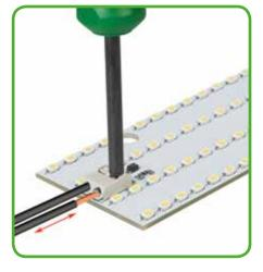
To connect stranded conductors, gently depress the push-button with the actuation tool to first open the spring. To release conductors, gently depress the push-button with the actuation tool.
