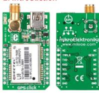
GPS Click - L10 is an accessory board in mikroBus<sup>TM</sup> form factor. It's a compact solution for adding GPS functionality to your device. It features Quectel® L10, high performance MTK positioning engine. GPS Click - L10 communicates with target board through UART or I<sup>2</sup>C interface. Data can be acquired using PC application through USB connection. Board features connector compatible with active and passive antennas. It can operate on 3.3V power supply only.
