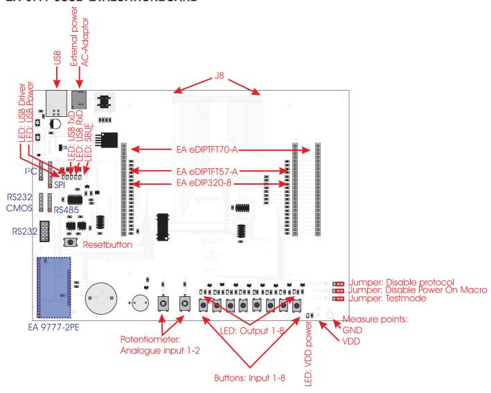
The Evaluation board provides a variety of features, starting with LEDs to indicate data-transfer, ending with potentiometers to use the analogue inputs of EA eDIPTFTs.
