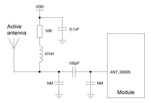
Figure 35: Reference Circuit of GNSS Active Antenna
