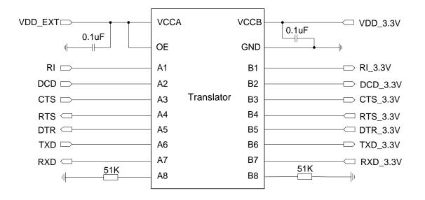
Figure 19: Reference Circuit with Translator Chip
