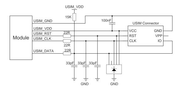
Figure 23: Reference Circuit of the 6 Pin USIM Card
