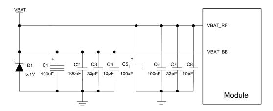
Figure 7: Star Structure of the Power Supply
