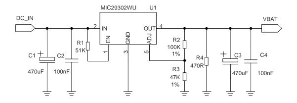
Figure 8: Reference Circuit of Power Supply
