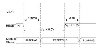
Figure 15: Timing of Resetting Module
