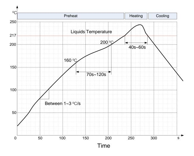
Figure 45: Liquids Temperature
