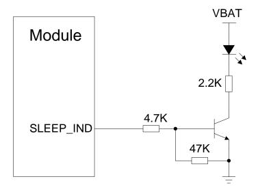
Figure 31: Reference Circuit of the SLEEP\_IND
