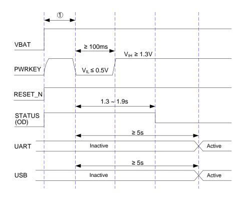
Figure 11: Timing of Turning on Module
