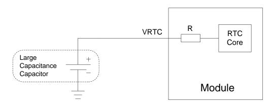
Figure 18: RTC Supply from Capacitor
