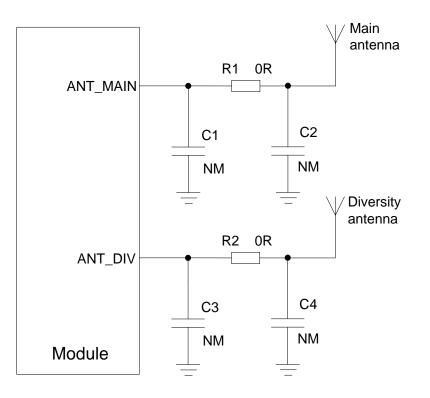
Figure 33: Reference Circuit of Antenna Interface
