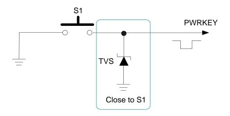
Figure 10: Turn on the Module Using Keystroke
