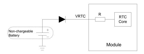
Figure 16: RTC Supply from Non-chargeable Battery
