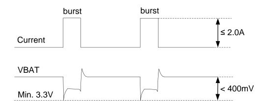
Figure 6: Voltage Drop during Transmitting Burst
