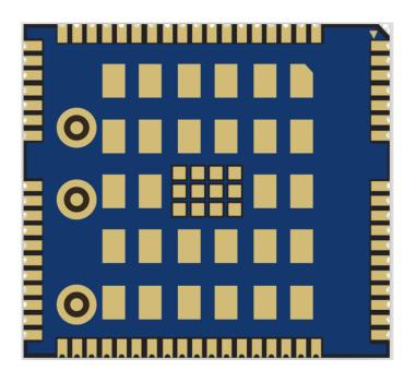
Figure 44: Bottom View of the Module
