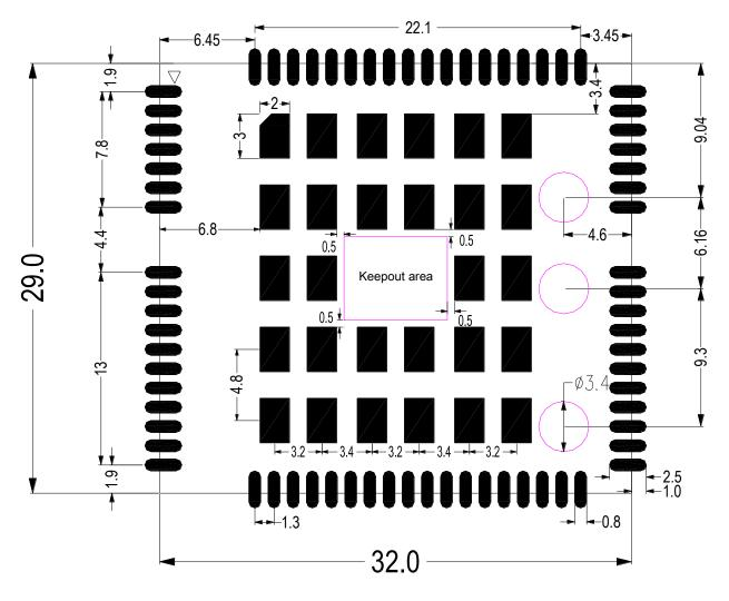
Figure 42: Recommended Footprint (Top View)
