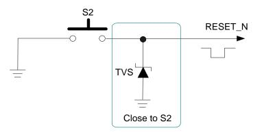
Figure 14: Reference Circuit of RESET\_N by Using Button
