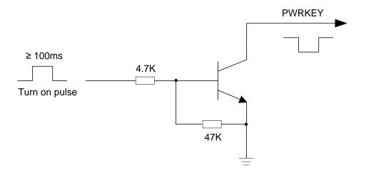
Figure 9: Turn on the Module Using Driving Circuit
