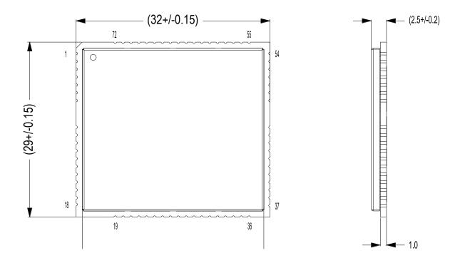
Figure 39: UC20 Top and Side Dimensions
