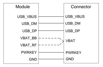
Figure 25: Test Points of Firmware Upgrade
