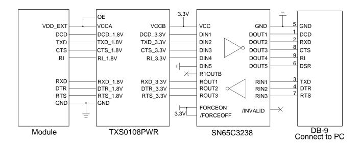
Figure 21: RS232 Level Match Circuit
