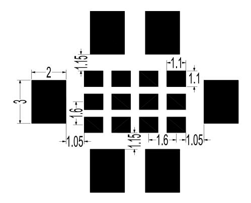
Figure 41: Bottom Pads Dimensions (Bottom View)
