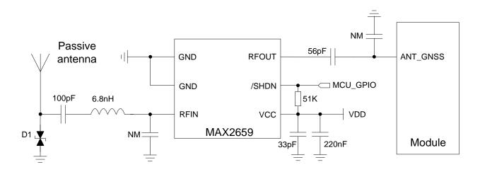
Figure 34: Reference Circuit of GNSS Passive Antenna
