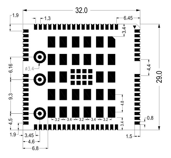
Figure 40: UC20 Bottom Dimensions (Bottom View)
