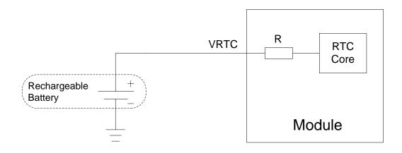
Figure 17: RTC Supply from Rechargeable Battery
