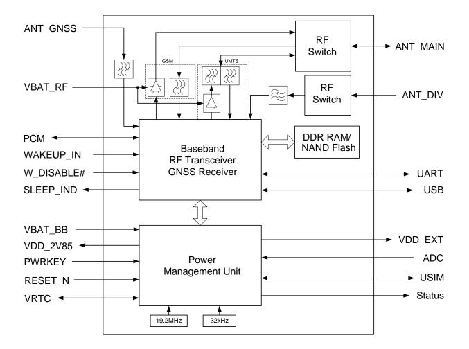
Figure 1: Functional Diagram
