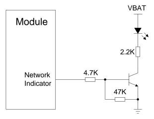
Figure 29: Reference Circuit of the Network Indicator
