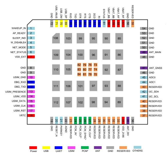
The following figure shows the pin assignment of the UC20 module.
