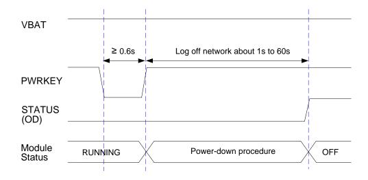
Figure 12: Timing of Turning off Module
