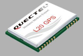
L20, a GPS receiver module, which is based on the lastest SIRF-starIV ROM version 2.2, features extremely compact profile of 16.0 x 12.2 x 2.4mm and low current consumption of only 36 mA during tracking. Highest sensitivity down to -163dBm for tracking satellites along with lowest Time-To-First-Fix fulfill the toughest requirements.
