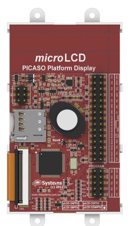
The µLCD-32WPTU has a 3.2" Wide TFT LCD display at the forefront of the design that showcases the power and capabilities of the PICASO processor. Combining a resolution of 240x400 pixels with 65K True to Life colours, the display module is perfect for animations, slideshows and other multimedia presentations.
