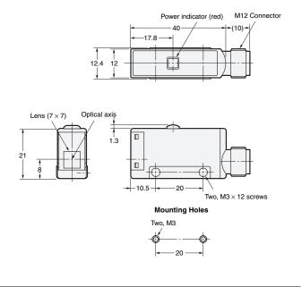
Note: Models numbers for Through-beam Sensors (E3S-AT\[]6) are for sets that include both the Emitter and Receiver.
