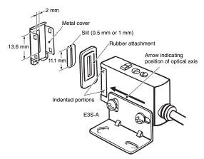
Apply the Slit to the lens of the Photoelectric Sensor marked with an arrow indicating the position of the optical axis (apply it to the bottom lens of Horizontal Sensors and the top lens of Vertical Sensors).
