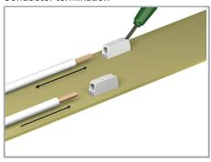
Insert fine-stranded conductors and remove all conductor types via operating tool. Solid conductors can also be terminated by simply pushing them in.
