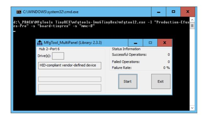
4 Press Start button (The iMX6 TinyRex board will boot firmware loaded over USB).
