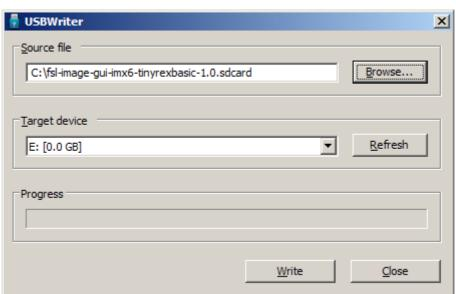
2 STEP Click on Write button and confirm a procedure.
