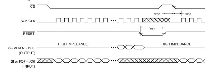
Note: The CS signal should be in the high state before the RESET signal is deasserted.
