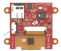
USER I/O – 15 way ZIF Socket 0.5mm pitch Upper Contact 8mm wide FPC Cable
