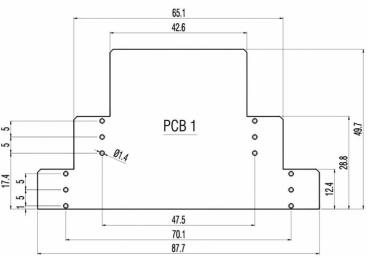
The CEM35 electronic housing is realized for connections up to 24 poles.
