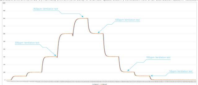
Test result: 0 ~ 1000ppm linear error <± 3%;
