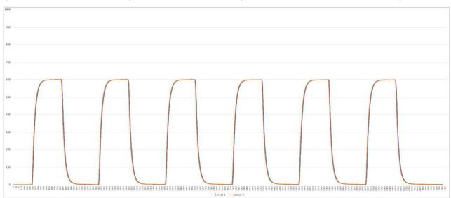
The test results show that the repeatability error range is <1ppm (1000ppm ± 1% of full scale is the normal range);
