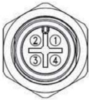
Pin Assignments Front View
