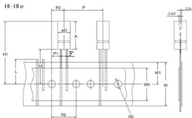
Size F means the distance after forming between the centers of the two lead pins.
