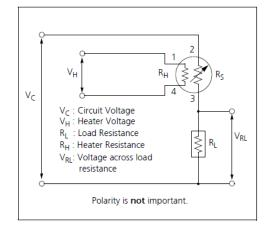
Fig 2. Standard circuit
