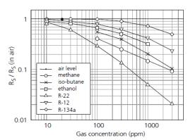
Fig3. Sensitivity characteristics
