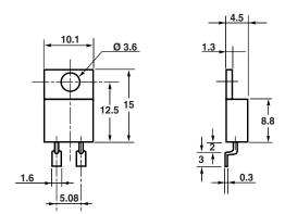
• Only for RTO 20 version C = during surface mount soldering temperature profile must not cause the metal tab of this device to exceed 220  $^\circ$ C.
