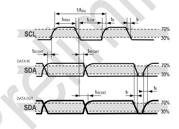
**Figure 4.** Timing diagram for digital input/output pads. SDA directions are seen from the sensor. Bold SDA lines are controlled by the sensor, plain SDA lines are controlled by the micro-controller. Note that SDA valid read time is triggered by falling edge of preceding toggle.
