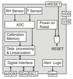
**Figure 1.** Functional block diagram of the SHT33-DIS. The CMOSens<sup>™</sup> technology allows providing for a fully calibrated I<sup>2</sup>C signal.
