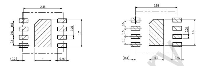
Figure 7. Recommended metal land pattern (left) and stencil apertures (right) for SHT33-DIS. The dashed lines represent the outer dimension of the DFN package. The PCB pads (left) and stencil apertures (right) are indicated through the shaded areas.
