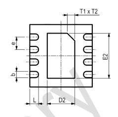
Figure 6. Dimensional drawing of SHT33-DIS sensor package.
