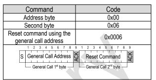
**Table 7.** Reset through the general call address (Clear blocks are controlled by the microcontroller, grey blocks by the sensor).
