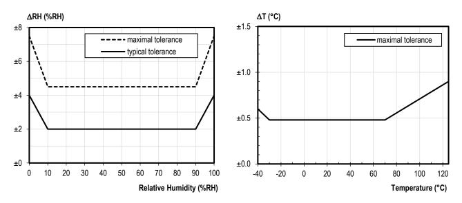
Figure 2. Maximal and typical tolerance of *RH* at 25°C and maximal tolerance for *T*.
