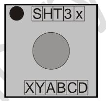
Figure 5. Top view of the SHT33-DIS illustrating the laser marking.
