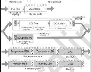
**Table 10.** Measurement commands in single shot mode. Thefirst "SCL free" block indicates a minimal waiting time of 1ms.(Clear blocks are controlled by the microcontroller, greyblocks by the sensor).
