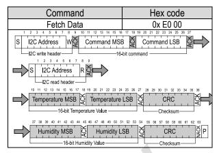
**Table 3.** Fetch Data command (Clear blocks are controlled by the microcontroller, grey blocks by the sensor).
