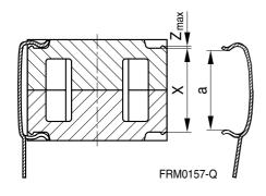
$F_{min}$ : Extension of clamp from a to  $a_2 = X_{min}$  $F_{max}$ : Extension of clamp from a to  $a_1 = X_{max}$
