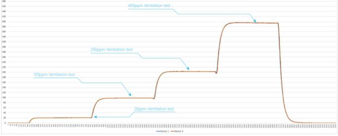
Test result: 0-200ppm linear error <± 3%; 200-500ppm linear error <± 5%;
