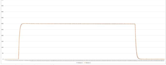
Test results: 2 hours ventilation, range drift <2ppm;
