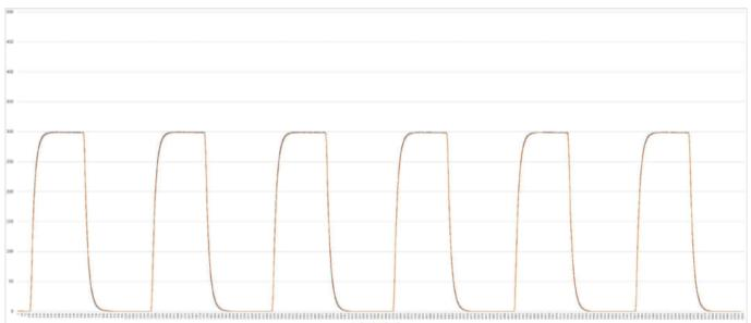
Temperature environment: 28°C ; Humidity environment: 55%; Air chamber space: 0.03m<sup>3</sup>; Gas flow of gas distribution system: 5000sccm;
