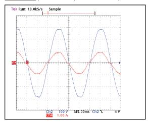
The pulsed input current of EC fans gives rise to current harmonics, which additionally increases the load on the supply network and causes greater losses as a result of reactive power.
