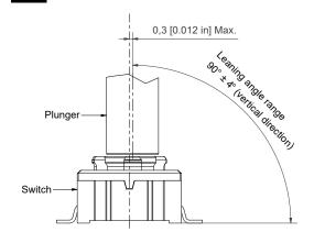
For the optimal performance of the switch use the recommended operating conditions.
