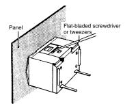
**Note:** Do not pry up the flange support more than necessary or the switch holding portions may be damaged.
