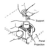
**Note:** Completely remove any burrs on the panel cutout surface; otherwise, the flange and Switch will not attach solidly.
