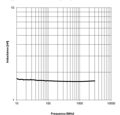
DESCRIPTION Projection **WE-CAIR Air coil** Würth Elektronik eiSos GmbH & Co. KG EMC & Inductive Solutions Max-Eyth-Str. 1 Order.- No. 74638 Waldenburg COMPLIANT SIZE Germany Tel. +49 (0) 79 42 945 - 0 744910016 www.we-online.com A4 2014-10-27 SSt 1.0 HBH eiSos@we-online.com REV BY Size: 1322 DATE CHECKED
