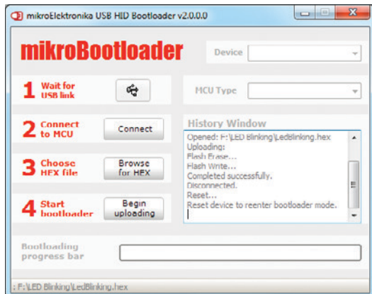
Figure 1-7: mikroBootloader ready for next job
