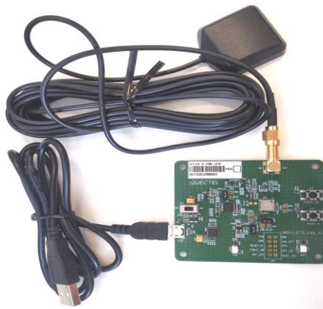
Figure 2: EVB and Accessories Assembly
