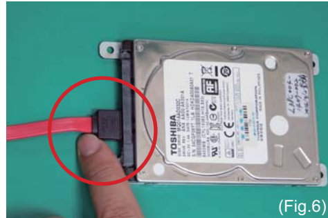
6. Connect the SATA DATA cable with HDD(Fig.6)
