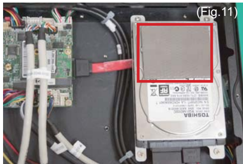
11. Attach the thermal pad on the HDD and avoid the heat-dissipating holes at the same time. (Fig.11)
