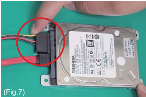
7. Connect the SATA Power cable with HDD. (Fig.7)
