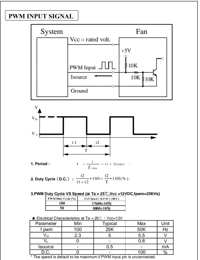
\* Min. start up duty cycle is 5%. Please don't apply 1 ~ 4% duty cycle to prevent unstable fan speed.
