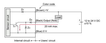
Note: The emitter does not incorporate the output.
