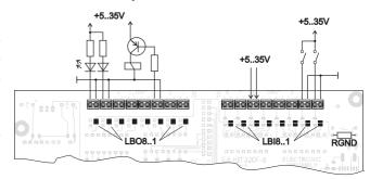
The collector and emitter of a transistor is brought out at the screw-type terminals as the output. Each output can switch a maximum of 10mA.
