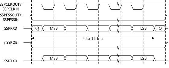
Figure 74. Motorola SPI frame format, single and continuous transfers, with SPO=1 and SPH=1, Q is an undefined signal.
