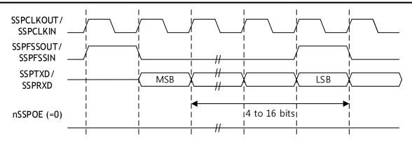
Figure 68. Texas Instruments synchronous serial frame format, continuous transfers
