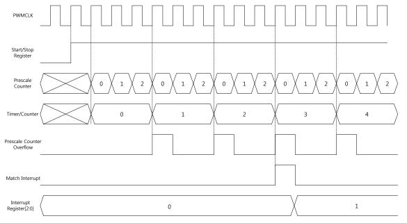
Figure 33 Timer/Counter timing diagram with match interrupt
