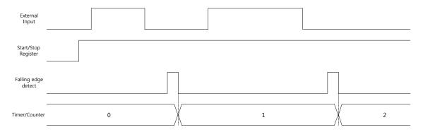
Figure 31 Counter mode with falling edge
