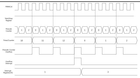
Figure 34 Timer/Counter timing diagram with overflow interrupt
