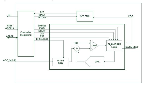
Figure 22. ADC block diagram
