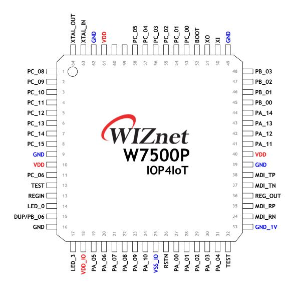
Figure 81 W7500P pin layout
