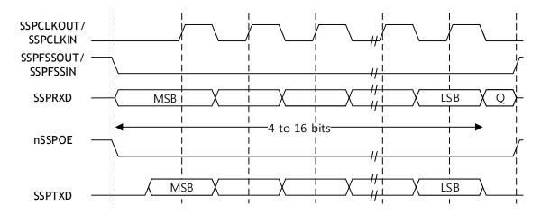
Figure 69 Motorola SPI frame format, single transfer, with SPO=0 and SPH=0
