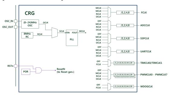
Figure 10 CRG block diagram
