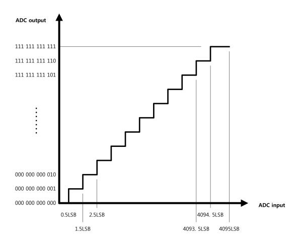
Figure 82. ADC transform function
