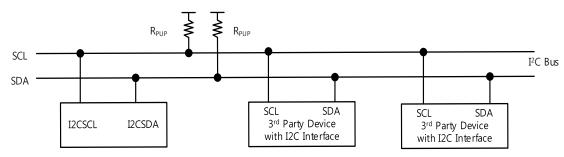
Figure 45. I2C Bus Configuration
