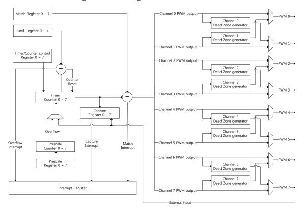
Figure 25 PWM block diagram
