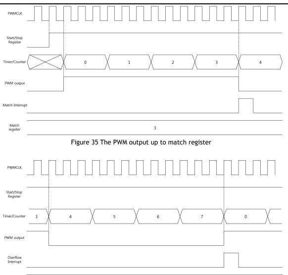
Figure 36 The PWM output up to limit register
