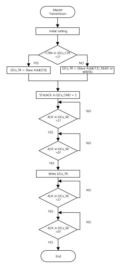
Figure 54. Master TRANSMIT with ADDR10=0 in the I2Cx\_CTR
