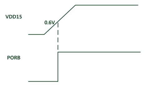
Figure 3 POR reset waveform
