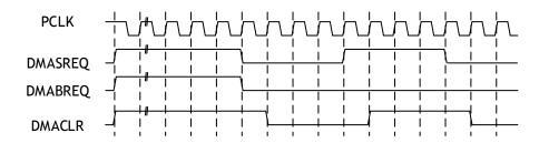
Figure 66. DMA transfer waveforms
