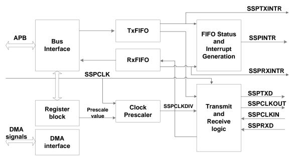
Figure 65. SSP block diagram
