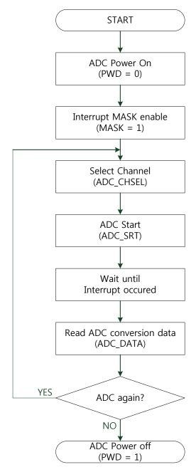
Figure 24. The ADC operation flowchart with interrupt
