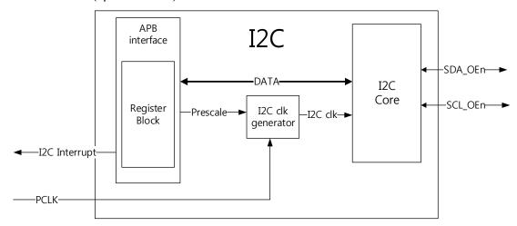
Figure 46. I2C block diagram
