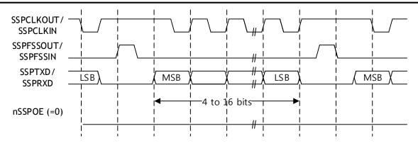
Figure 73. Motorola SPI frame format, continuous transfers, with SPO=1 and SPH=0
