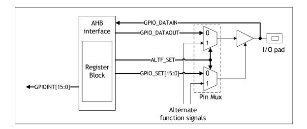
Figure 16. GPIO block diagram
