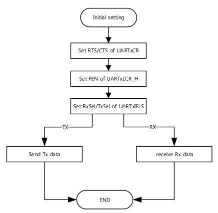
Figure 61. Transmit and Receive data flow chart
