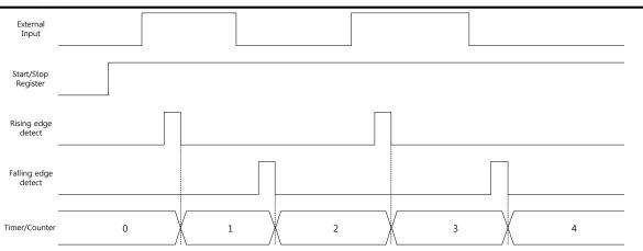
Figure 32 Counter mode with rising and falling edge
