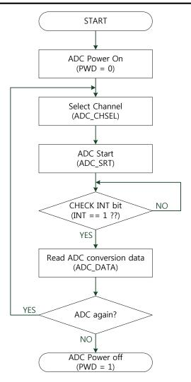
Figure 23. The ADC operation flowchart with non-interrupt
