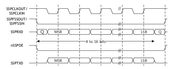
Figure 74. Motorola SPI frame format, single and continuous transfers, with SPO=1 and SPH=1
