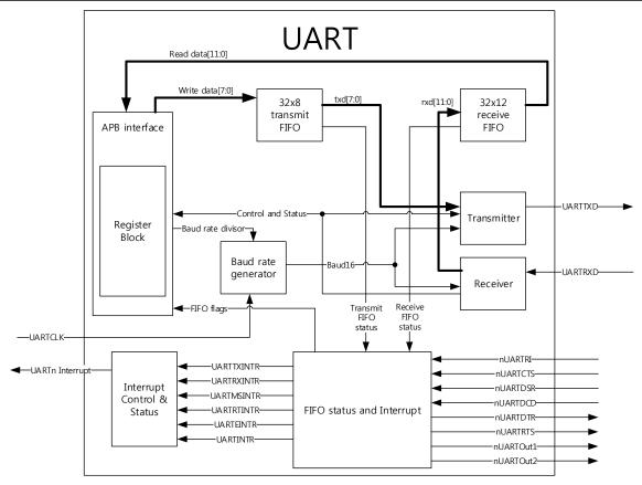
Figure 57. UARTO,1 Block diagram
