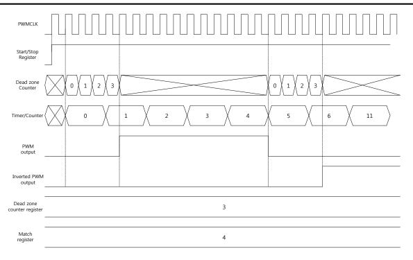
Figure 38 PWM waveform with dead zone counter
