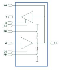
Figure 15. function schematic of digital/analog mux IO pad
