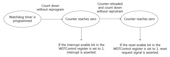
Figure 44 Watchdog timer operation flow diagram
