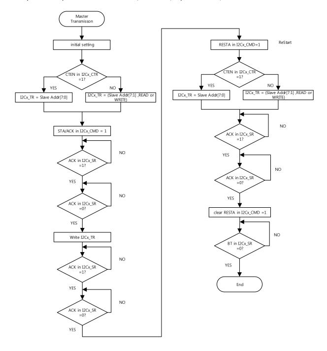
Figure 55. Master Transmit with Repeated START
