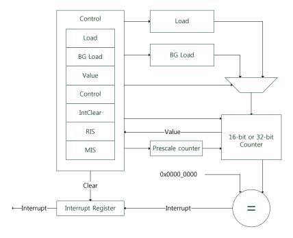
Figure 42 Block diagram of Dualtimer
