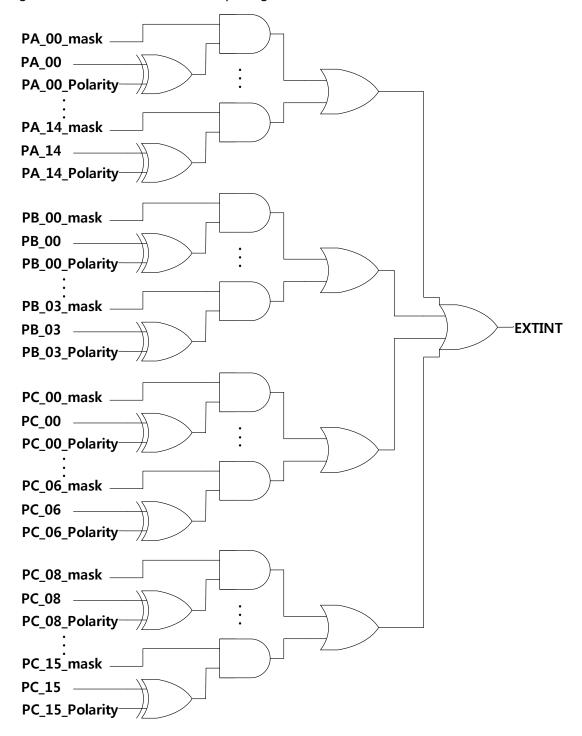
Figure 13. External Interrupt diagram
