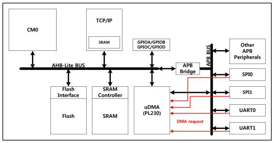
Figure 20. DMA Block diagram
