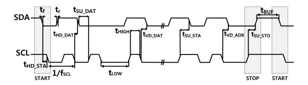
Figure 83. I2C bus AC waveform
