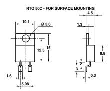
Only for RTO 50 version C = during surface mount soldering, the soldering temperature profile must not cause the metal tab of this device to exceed 220 °C.
