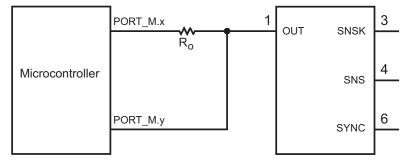
Electromechanical devices like relays will usually ignore the short HeartBeat pulse. The pulse also has too low a duty cycle to visibly affect LEDs. It can be filtered completely if desired, by adding an RC filter to the output, or if interfacing directly and only to a high-impedance CMOS input, by doing nothing or at most adding a small noncritical capacitor from OUT to Vss.
