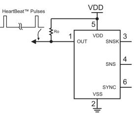
If the sensor is wired to a microcontroller as shown in Figure 3-7 on page 11, the microcontroller can reconfigure the load resistor to either Vss or Vdd depending on the output state of the QT1011, so that the pulses are evident in either state.
