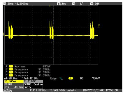
Figure 5-1. T<sub>G2</sub> – Time Between Bursts (LP Mode)
