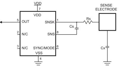
Note: A bypass capacitor should be tightly wired between Vdd and Vss and kept close to pin 7.
