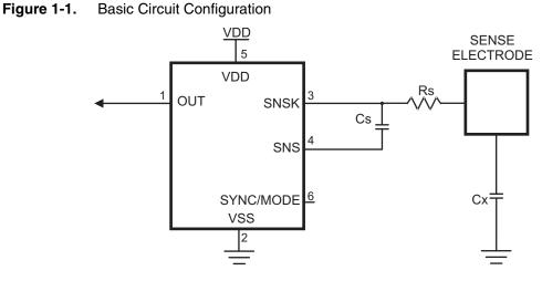
Note: A bypass capacitor should be tightly wired between Vdd and Vss and kept close to pin 5.
