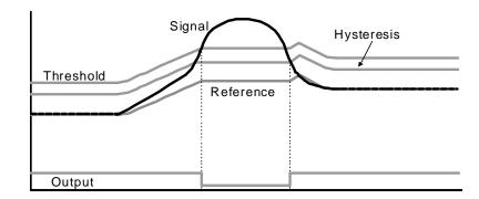
Figure 3-5. Drift Compensation
