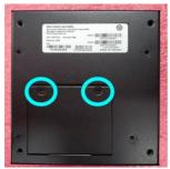
**Step 6.** Place the top cover and secure with screws.
