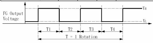
$T=\begin{array}{c} T1+T2+T3+T4=1 & Rotation \\ T=\begin{array}{c} 60 \\ \hline rpm \end{array}$
