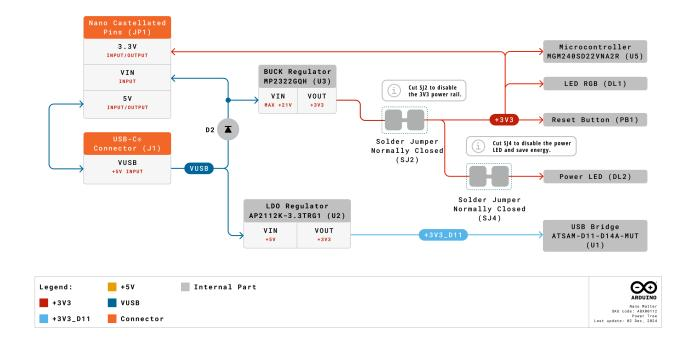
**Low-Power Tip:** For power efficiency, safely cut the LED jumper and connect an external +3.3 VDC power supply to the board's 3V3 pin. This configuration does not power the board's USB bridge.
