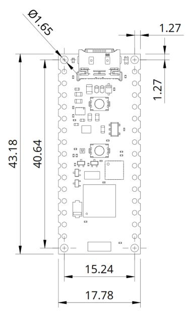
The Nano Matter has four 1.65 mm drilled mounting holes for mechanical fixing.
