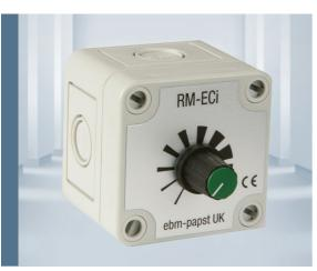
The RM-ECi controller is for use with the full range of ebm-papst EC fans. Powered by the 10VDC output from the motor, it provides infinitely variable, manual speed control between 0% and 100%.
