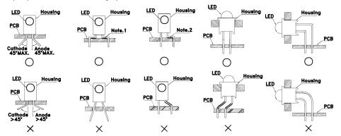
" $\bigcirc$ " Correct mounting method " $\times$ " Incorrect mounting method
