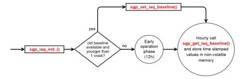
Call sgp\_iaq\_init...() to reset all SGP baselines. After the accelerated warm-up phase (see 3.9. for durations), the initialization takes 20 seconds, during which sgp\_iaq\_measure() output will not change.
