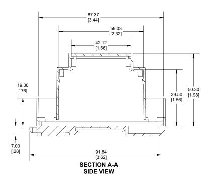
Enclosures can be Factory Modified (Milling, Drilling, Printing etc.) Contact Factory (modshop@hammfg.com) for quotes Solid models of this enclosure available in .stp or .x\_t (Part number and text placement/orientation on our products are subject to change, we do not recommend using them as a locating reference for modification purposes)
