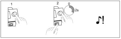
Via a rotary motion and respective pushing, the station can be configured or newly recorded with the factory settings.
