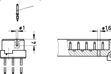
To avoid cross-plugging of adjacent connectors a coding system is required. Drill out the male connector at pre-centered point according to the sketch. Use the setting tool 09 99 000 0103 to insert the coding pin 09 06 000 9950 into the existing hole in the female connector.
