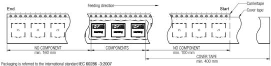
Projection 3.5 SSt 2014-09-16 BD 3.4 2013-12-11 SSt SSt SSt 3.3 2013-04-29 SSt Würth Elektronik eiSos GmbH & Co. KG EMC & Inductive Solutions 3.2 SSt SSt 2012-12-05 Max-Eyth-Str. 1 3.1 2012-10-25 SSt BD 74638 Waldenburg Germany Pull-of force 3.0 2012-09-03 SSt BD Tel. +49 (0) 79 42 945 - 0 Tape width | 16 mm | 0,1 N - 1,3 N www.we-online.com 2.0 ME 2008-01-01 Tape width | 24 mm | 0,1 N - 1,3 N eiSos@we-online.com BY CHECKED
