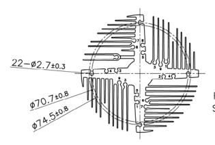
For LED Module Assembly Screw torque max 12kgf.cm
