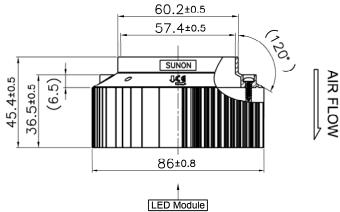
Assembly direction of customer's LED Module
