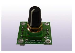
**General remarks:** The CN1003 controller is designed for use with the full range of ebm-papst ECi (Electronically Commutated with integrated electronics) fans, it is powered via the DC output from by the fan and provides a 0-10V signal to enable infinitely variable speed control. The controller also enables speed measurement of the fan using a multimeter with a frequency measuring facility (where a tacho output is provided from the fan).
