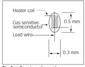
Fig 1a. Sensing element
