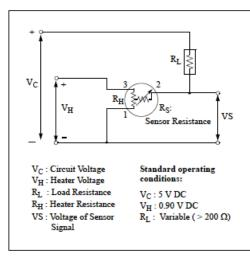
Fig 3. Standard circuit
