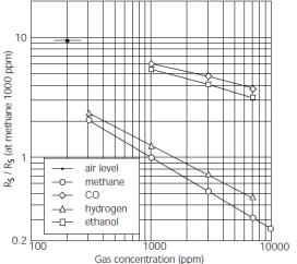
Fig4. Sensitivity characteristics SB12C00E 181001V1
